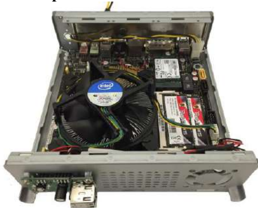
Figure 8 – Computer case with Cover Removed
