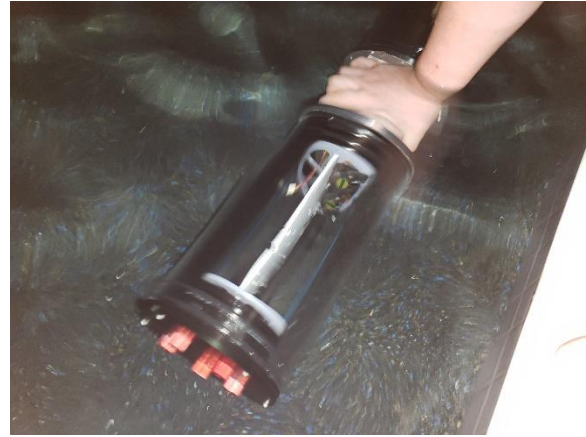
Figure 2: The electronics enclosure was leak tested separately from the rest of the chassis. It was pushed down under the surface of the water and monitored for any potential leaks.
